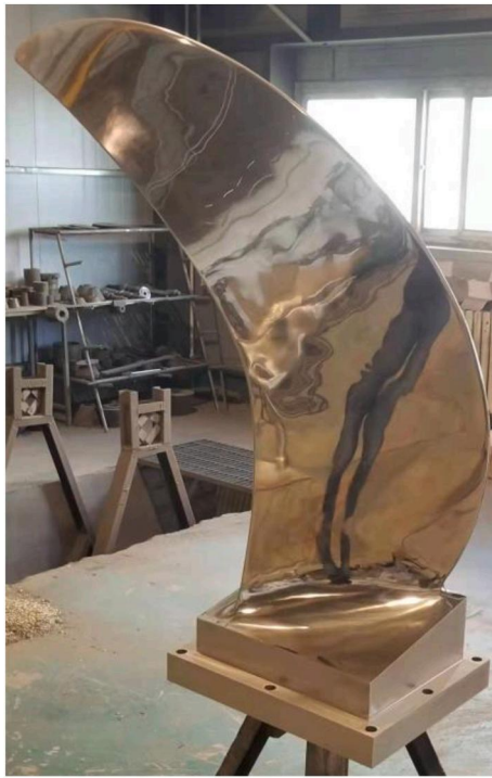
Fig. 5. E1619 blades and casting site.
