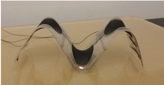
Fig. 4 Flapping wing system formed from joining three DEMES rotary joints together
