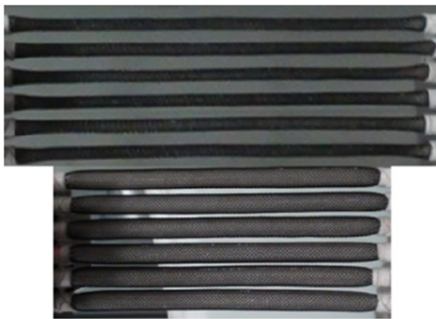
Figure 4. Depiction of six PMFs in the resting length (0 MPa) and in the free contraction state (0.35 MPa).
