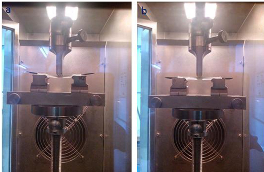
Fig. 3. Three-point bending test procedure at A_f + 22 K.
