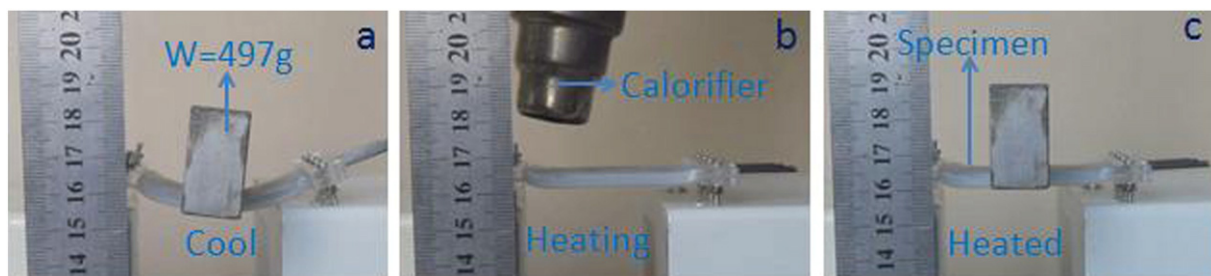
Fig. 9. Demonstration of the varying stiffness capability of SMA-elastomer composites.
