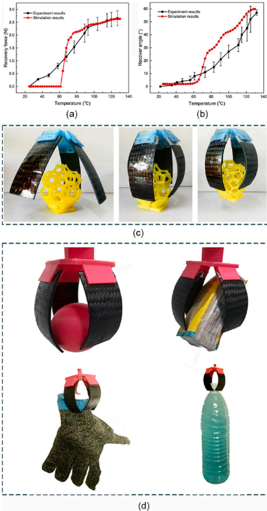
Fig. 5. Test of target grip performance. (a) Recovery force and (b) recovery angle of single gripper (c) Functionality test of target capture and movement. (d) Adaptability test.
