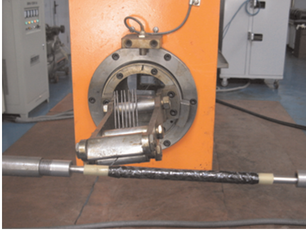
Figure 4. Filament wound of the F 2 MC tube.
