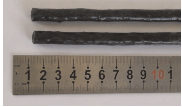
Figure 5. The F 2 MC tube specimens.
