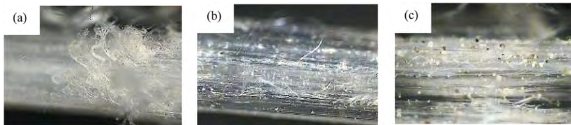
Fig. 11. Synthetic fibre surface after bond strength tests: (a) plain fibre (uncoated), (b) PU resin-coated fibre and (c) UF resin-coated fibre [79].
