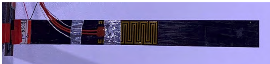
Fig. 11. Physical picture of SMPC specimen with electrothermal film.
