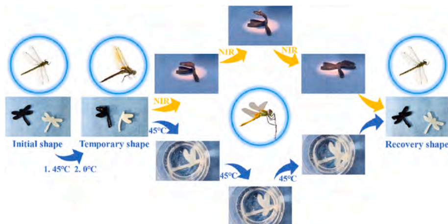
Fig. 7. Shape memory performances of bionic dragonfly hydrogels.
