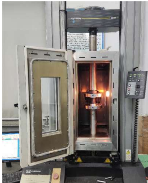
Fig. 10. The axial compressive tests of SMPC cylindrical shells.
