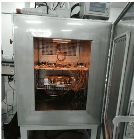
Figure 16 Thermal cycling test in air of the SMPC-FSAS flight hardware.
