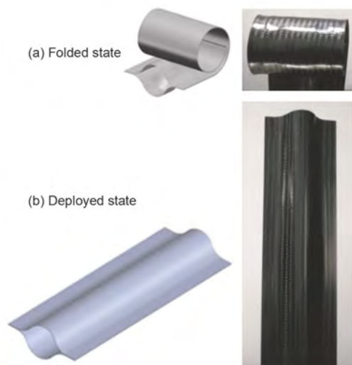
Figure 5 (Color online) The design of SMPC variable-stiffness tubes with lenticular cross section. (a) Folded state; (b) deployed state.
