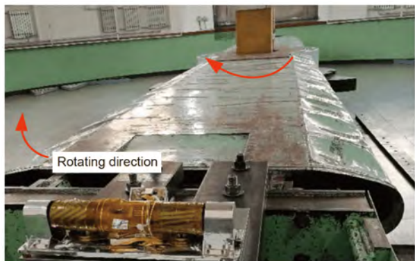
Figure 10 (Color online) Setup of acceleration test in X direction for the SMPC-FSAS flight hardware.
