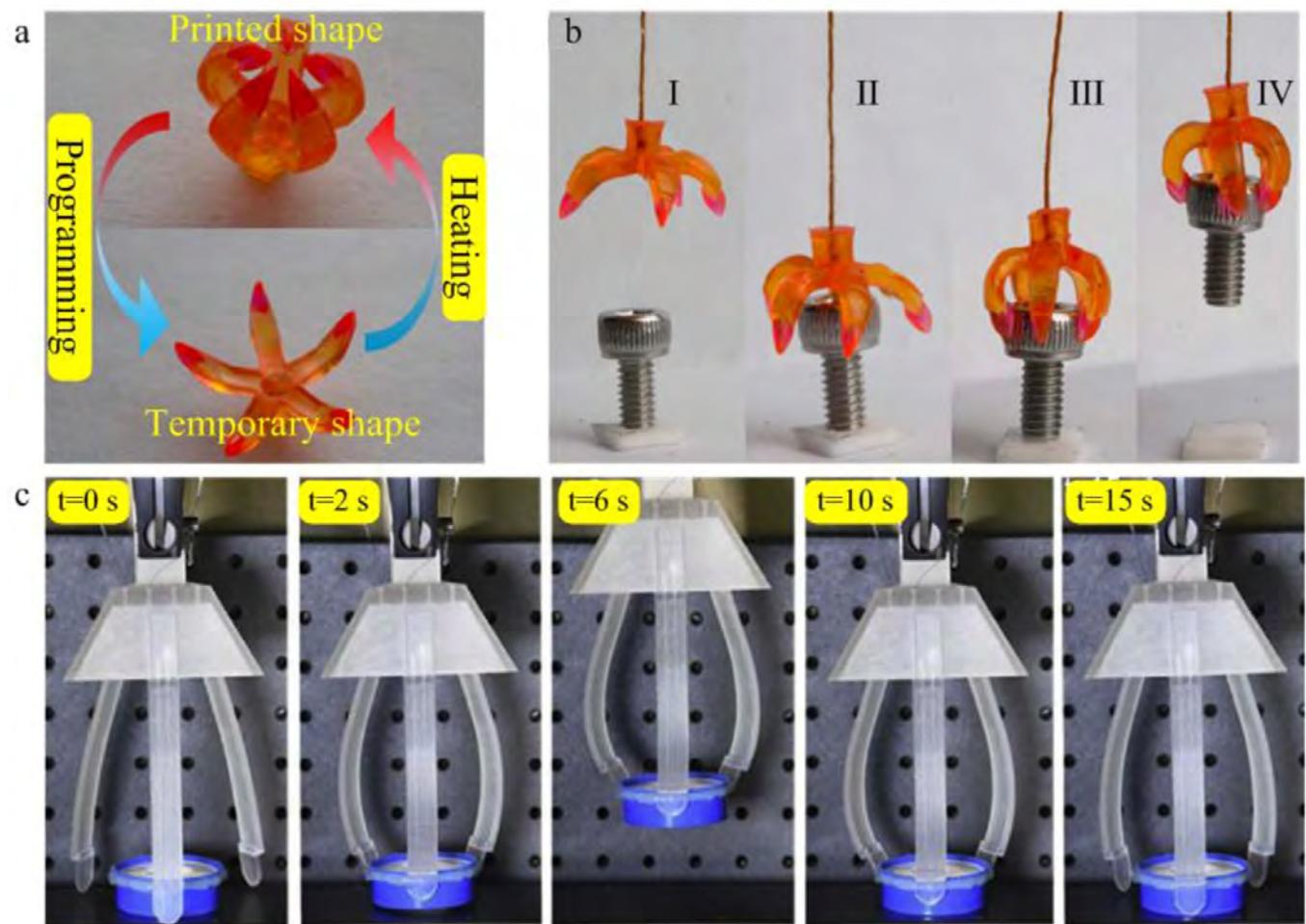
**Figure 13.** 4D printed multi-material smart grippers. (a) Photographs of the fabricated smart gripper showing the transition from the temporary to the permanent shape and vice versa, (b, i–iv) snapshots showing the process of gripping an object [65], and (c) snapshots showing the process of grasping and releasing of a 15 g cylindrical object by the smart gripper in a span of 15 s (reprinted with permission from [92]. Copyright (2019) Elsevier).
