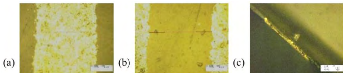
Fig. 6. Optical micrographs. (a) Line width, (b) separation, (c) thickness.
