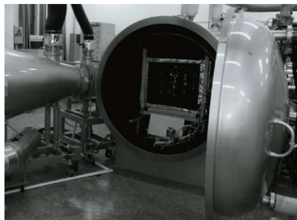
Figure 13 Thermal equilibrium test: solar simulator and the SMPC-FSAS flight hardware mounted on the simulated plate.
