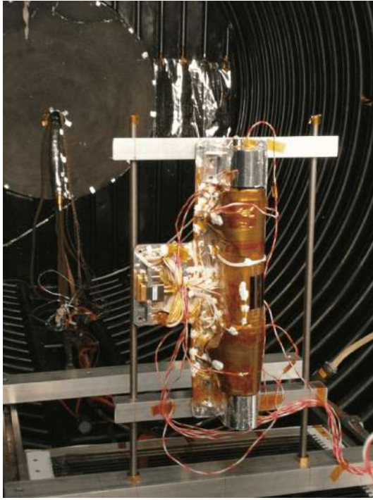
Figure 15 Setup of thermal vacuum cycling test of SMPC-FSAS flight hardware.
