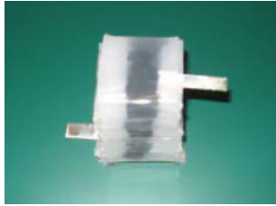
Fig. 2. Folded dielectric elastomer actuator.
