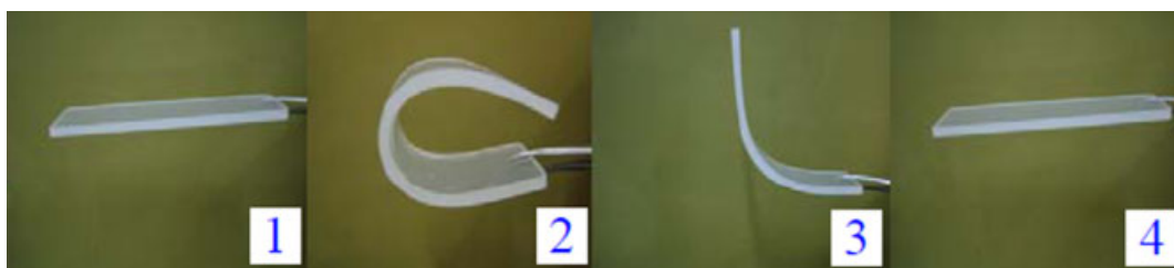
Figure 7. Series of photographs showing the macroscopic shape-memory effect of pure SMP matrix.
