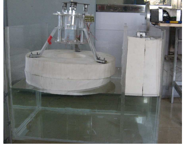
Fig. 8: (Color online) Experimental setup for the energy harvester based on the silicone dielectric elastomer.
