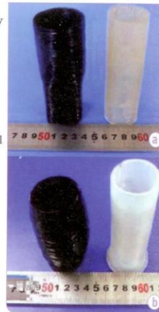
Fig. 6: Carbon fibre reinforced composite parts and the corresponding mandrels a) Multi-shaped parts b) Bottle-shaped parts
