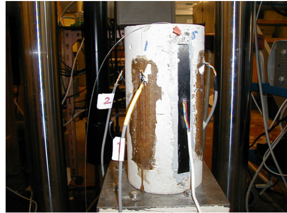
Figure 15. Photograph of a concrete cylinder with a CFRP-based SSPS.
