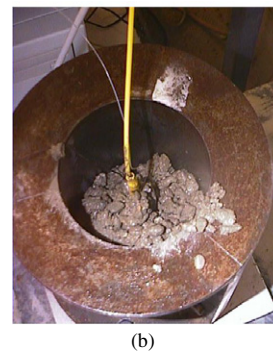
Figure 11. Compression testing of a concrete cylinder with an ESPS. (a) Schematic illustration. (b) Photograph during the pouring stage.
