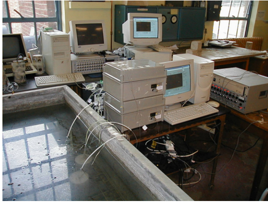
Figure 6. Photograph of experimental set-up for cure monitoring of concrete cylinders.
