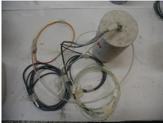
Figure 7. Concrete cylinder with embedded sensors.
