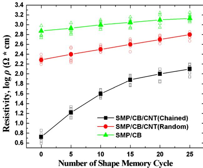
FIG. 5. (Color online) Degradation of electrical conductivity upon shape memory cycles.
