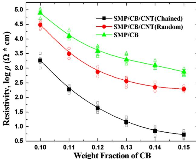
FIG. 3. (Color online) Curves of resistivity vs weight fraction of CB.
