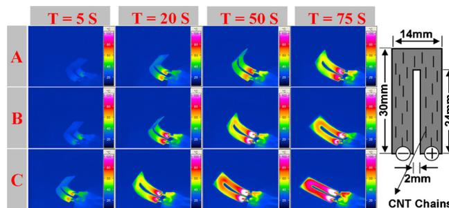
FIG. 4. (Color online) Snap shots of shape recovery and temperature distributions. Sample A: SMP/CB, Sample B: SMP/CB/CNT (random), Sample C: SMP/CB/CNT (chained). Right figure shows the sample dimension and experimental setup for Sample C.
