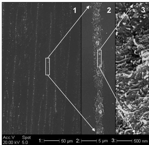
FIG. 1. SEM image of SMP/CB/CNT (chained) with 10 wt % CB. Insets: zoom-in views of one CNT chain.
