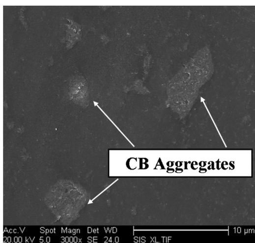
FIG. 2. SEM image of SMP composite filled with 10 wt % CB prepared under electric field.
