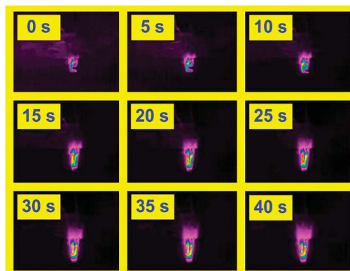
Fig. 7 Snap shots of shape recovery and temperature distributions of SMP nanocomposite incorporated with 0.6 g carbon fibers and 0.2 g carboxylic acid-functionalized CNTs.
