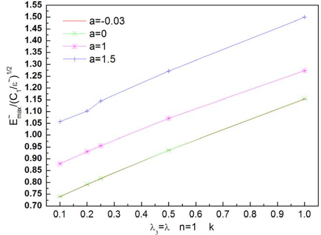
Figure 10. The critical nominal electric field when electrostriction coefficient  $r$  takes different values under the loading condition  $\lambda_3 = \lambda$ .
