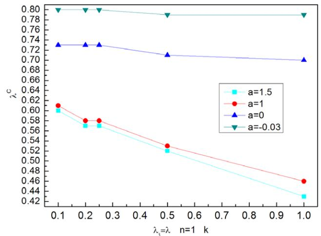
Figure 11. The critical stretch ratio when electrostriction coefficient  $r$  takes different values under the loading condition  $\lambda_3 = \lambda$ .
