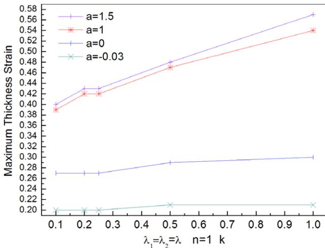
Figure 9. The critical thickness strain when electrostriction coefficient  $r$  takes different values under the loading condition  $\lambda_1 = \lambda_2 = \lambda$ .
