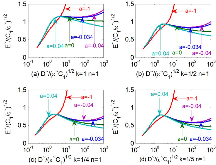
**Figure 2.** Relationship between the nominal electric displacement and the nominal electric field of dielectric elastomers for various values of  $r$  and  $k$ , under stretches that are biaxially equal  $\lambda_1 = \lambda_2 = \lambda$  (a)  $k = 1$ , (b)  $k = 1/2$ , (c)  $k = 1/4$ , (d)  $k = 1/5$ .
