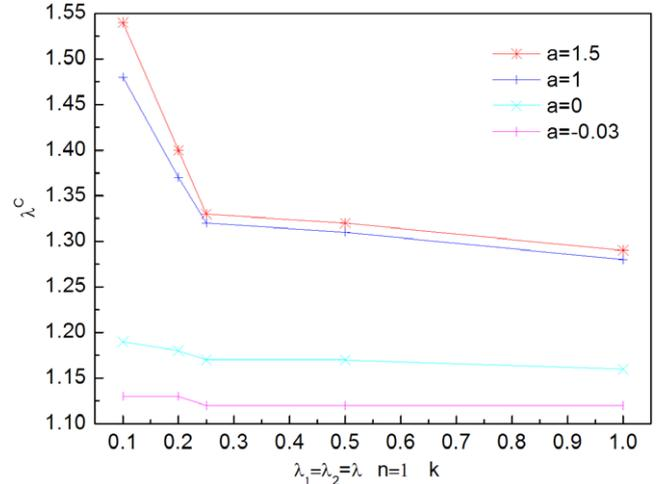
**Figure 7.** The critical stretch ratio when electrostriction coefficient  $r$  takes different values under the loading condition  $\lambda_1 = \lambda_2 = \lambda$ .
