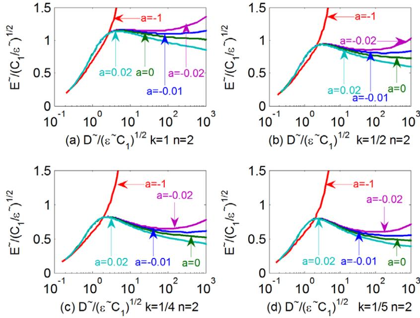
**Figure 4.** Relationship between the nominal electric displacement and the nominal electric field of dielectric elastomers for various values of  $r$  and  $k$ , under stretches that are biaxially equal  $\lambda_3 = \lambda$  (a)  $k = 1$ , (b)  $k = 1/2$ , (c)  $k = 1/4$ , (d)  $k = 1/5$ .
