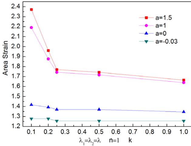
Figure 8. The critical area strain when the electrostriction coefficient  $r$  takes different values under the loading condition  $\lambda_1 = \lambda_2 = \lambda$ .
