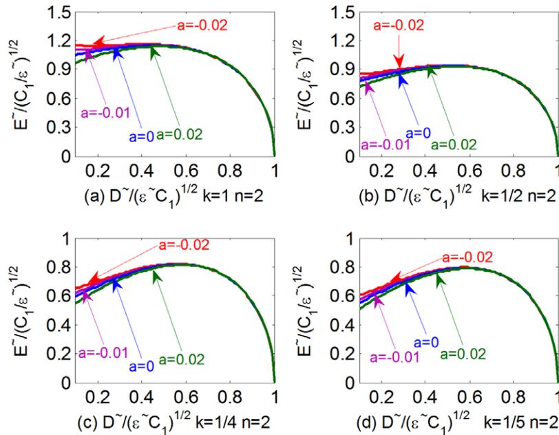
**Figure 5.** Relationship between the stretch ratio and the nominal electric field of different dielectric elastomers with different values of  $r$  and  $k$ ,  $\lambda_3 = \lambda$  (a)  $k = 1$ , (b)  $k = 1/2$ , (c)  $k = 1/4$ , (d)  $k = 1/5$ .
