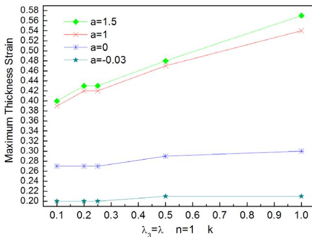
**Figure 13.** The critical thickness strain when electrostriction coefficient  $r$  takes different values under the loading condition  $\lambda_3 = \lambda$ .
