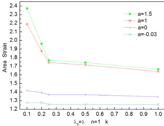
**Figure 12.** The critical area strain when the electrostriction coefficient  $r$  takes different values under the loading condition  $\lambda_3 = \lambda$ .
