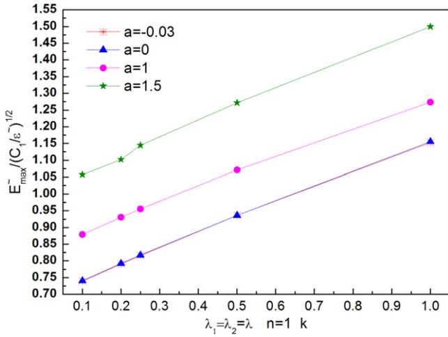
**Figure 6.** The critical nominal electric field when electrostriction coefficient  $r$  takes different values under the loading condition  $\lambda_1 = \lambda_2 = \lambda$ .
