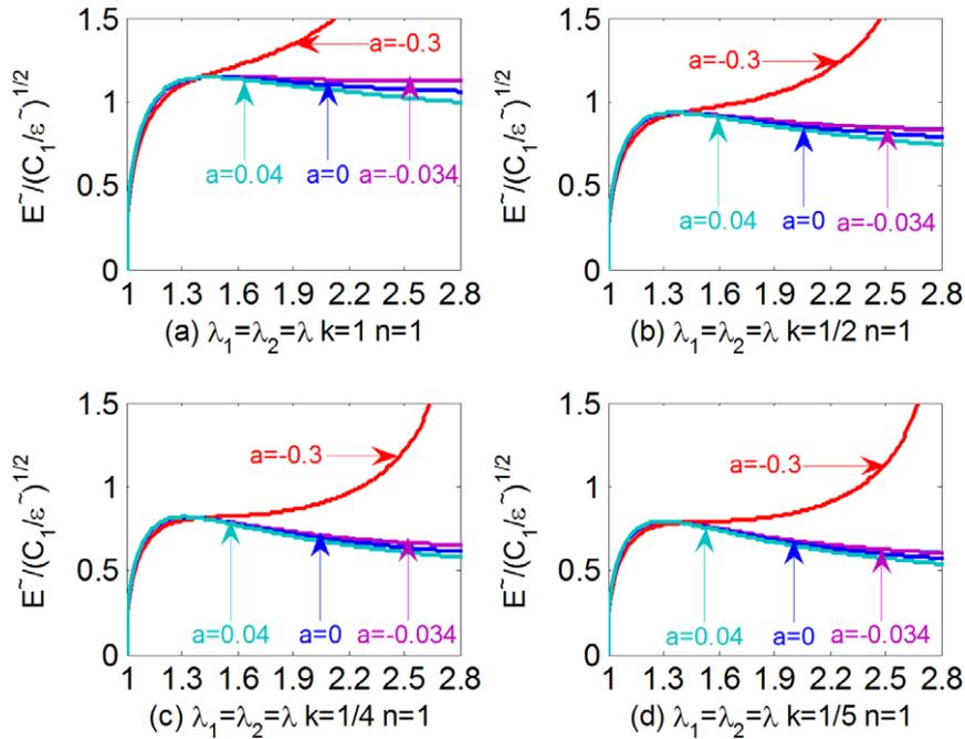
**Figure 3.** Relationship between the stretch ratio and the nominal electric field of different dielectric elastomers with different values of  $r$  and  $k$ , under stretches that are biaxially equal  $\lambda_1 = \lambda_2 = \lambda$  (a)  $k = 1$ , (b)  $k = 1/2$ , (c)  $k = 1/4$ , (d)  $k = 1/5$ .
