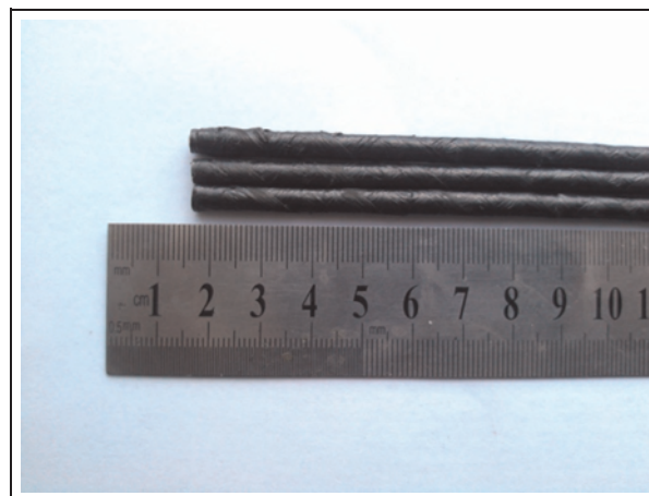
Figure 2. SMPC tube specimens. SMPC: shape memory polymer composite.
