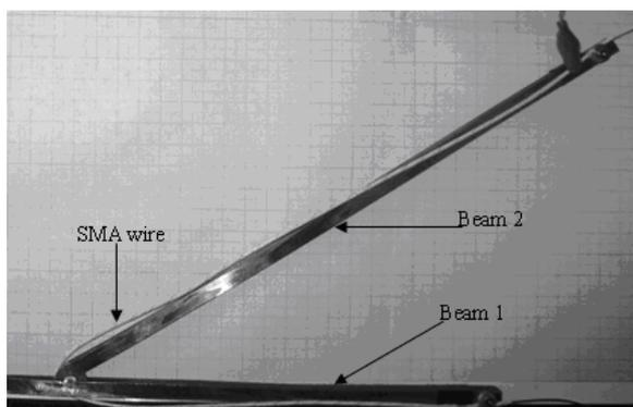
Fig.4 The SMA deployment hinge
