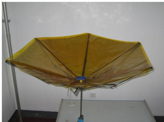
Fig.1 Deployable Antenna Actuated by Shape Memory Alloy Hinge
