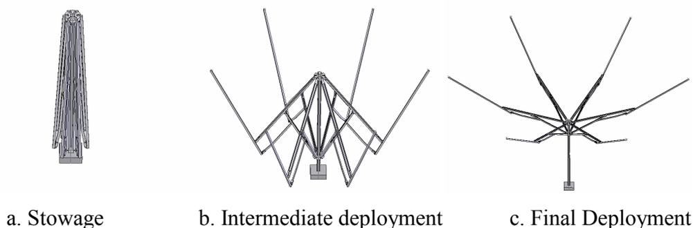
Fig.2 Process of deployment for the deployment truss
