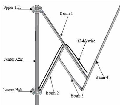
Fig.3 Deployable rib element for truss
