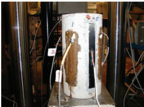
**Fig.19** Photograph of concrete cylinder with CFRP-based SSPS
