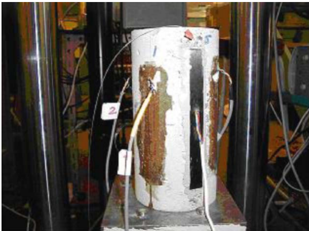
Fig. 18. Photograph of concrete cylinder with CFRP-based SSPS.
