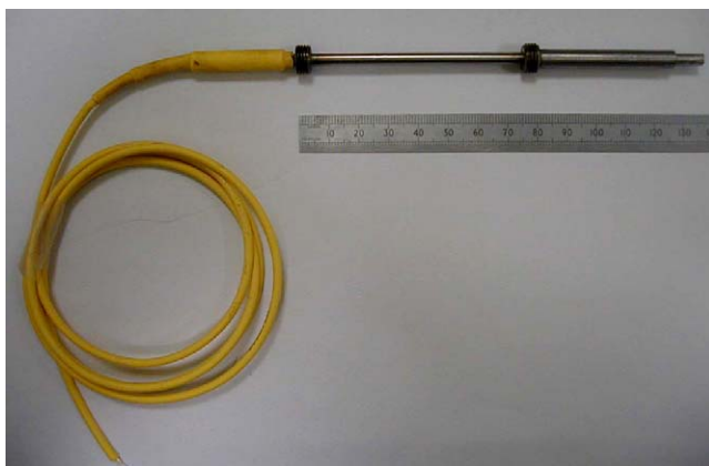
Fig. 2. Photograph of the steel tube-based ESPS.
