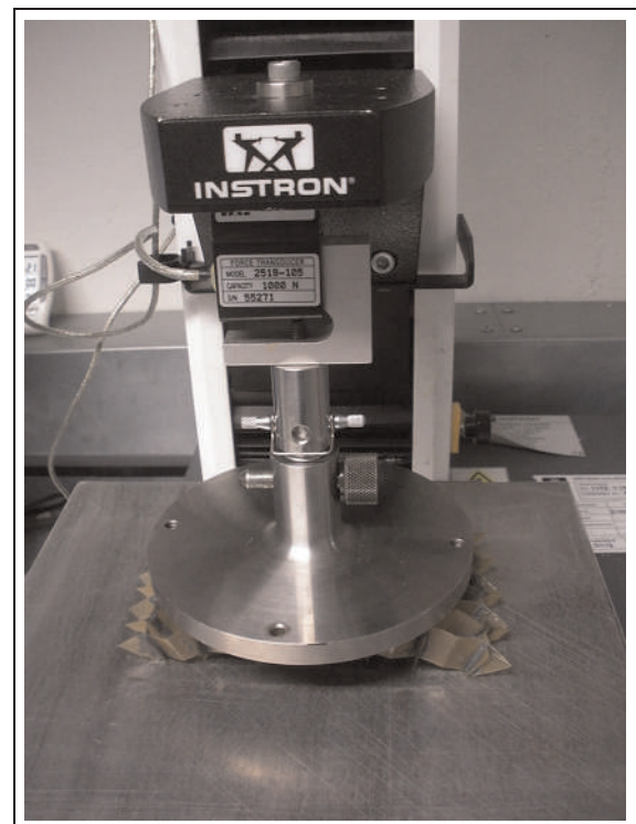
Figure 6. Curved SILICOMB sample experimental setup.
