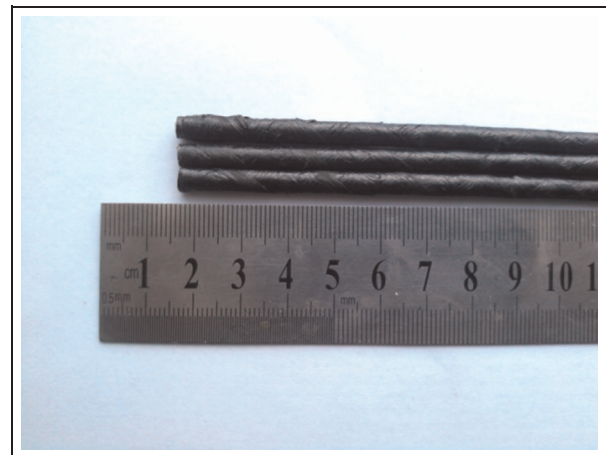
Figure 2. SMPC tube specimens. SMPC: shape memory polymer composite.
