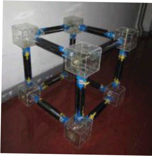
Figure 5. The simplified cubic deployable support structure.
