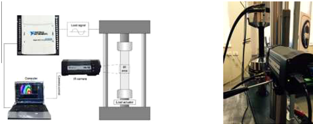
Fig. 4. Thermo-elastic stress analysis (TSA) testing setup.
