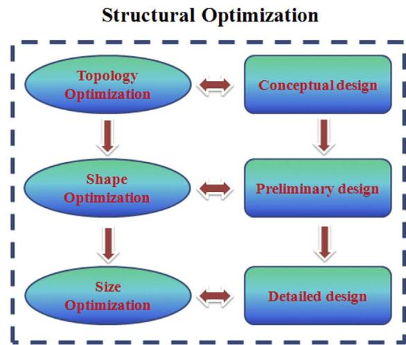
Fig. 1. Optimization methods for different structural design stages.
