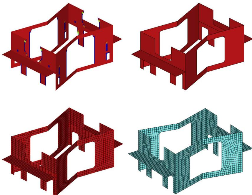
Fig. 9. Result of the multi-stiffness topology optimization with relative density  $\rho \geq 0.3$  (left) and the new design according to the optimized result (right).
