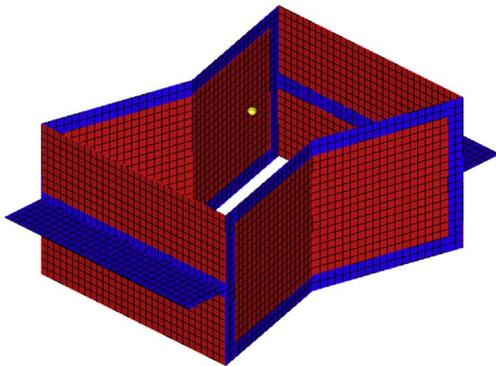
Fig. 4. The FE model used in the topology optimization process with the design domain (red), the non-design domain (blue) and a master node on the top surface. (For interpretation of the references to colour in this figure legend, the reader is referred to the Web version of this article.)
