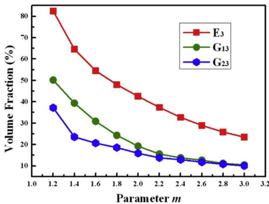
Fig. 8. vol fraction of the design domain for the optimized results VS the constraint's parameter  $m$ .
