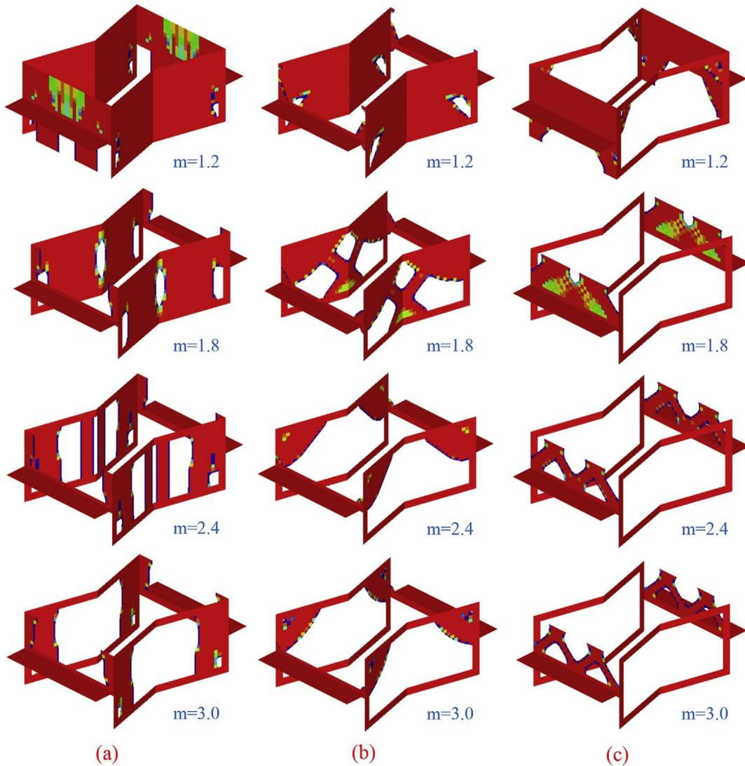
Fig. 7. Topology of the optimized results VS the constraint's parameter  $m$ : (a) flatwise compressive modulus  $E_3$ ; (b) transverse shear modulus  $G_{13}$ ; (c) transverse shear modulus  $G_{23}$ .
