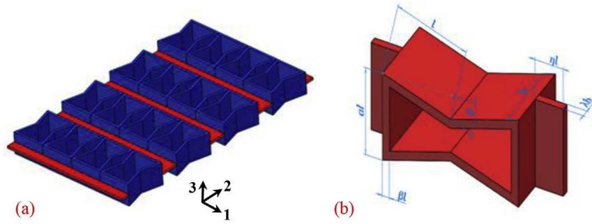
Fig. 3. Layout of the zero Poisson's ratio cellular structures (a); the geometry of a unit cell (b).
