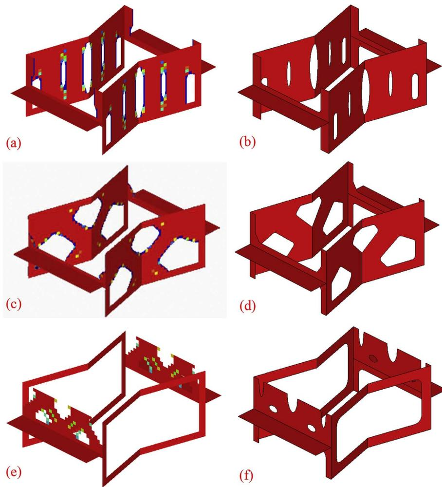
Fig. 5. Results of the single-stiffness topology optimization with elements' density  $\rho \geq 0.3$  and the new designs according to the optimized results: (a) and (b), flatwise compressive modulus  $E_3$ ; (c) and (d), transverse shear modulus  $G_{13}$ ; (e) and (f), transverse shear modulus  $G_{23}$ .
