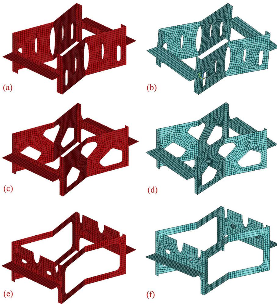
Fig. 6. Finite element models of the HyperWorks (red) and ANSYS (blue) analyses used to validate the out-of-plane mechanical performances of the new designs: (a) and (b), flatwise compressive modulus  $E_3$ ; (c) and (d), transverse shear modulus  $G_{13}$ ; (e) and (f), transverse shear modulus  $G_{23}$ . (For interpretation of the references to colour in this figure legend, the reader is referred to the Web version of this article.)
