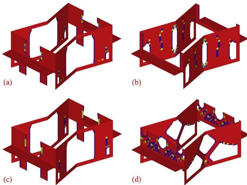
Fig. 11. Geometrical shape of the multi-stiffness topology optimization vs varying weighting coefficients: (a)  $w_3 = 0.34$ ,  $w_1 = w_2 = 0.33$ ; (b)  $w_3 = w_1 = 0.5$ ,  $w_2 = 0$ ; (c)  $w_3 = w_2 = 0.5$ ,  $w_1 = 0$ ; (d)  $w_3 = 0$ ,  $w_1 = w_2 = 0.5$ .
