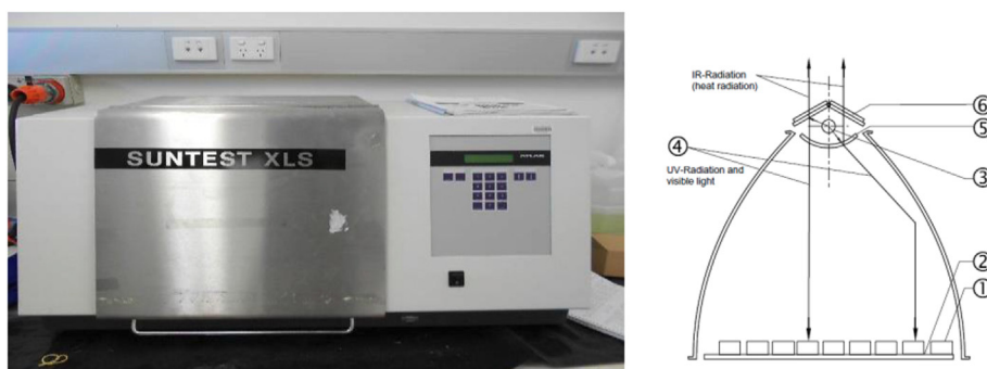
Fig. 2. SUNTEST XLS UV equipment, and schematic of the UV light chamber showing the components of the equipment 1. Specimens, 2. Sample table, 3. Xenon lamp, 4. Radiation, 5. Optical filter, 6. Mirror.
