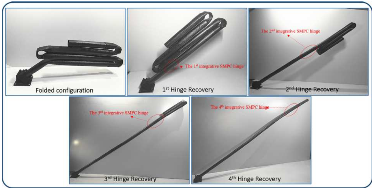
Fig. 24. Shape memory recovery process of self-deployable structure.
