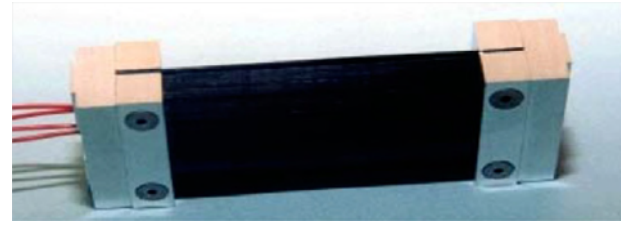
Figure 4. The early SMPC hinge prototype. Reused from [154] with permission from the authors.
