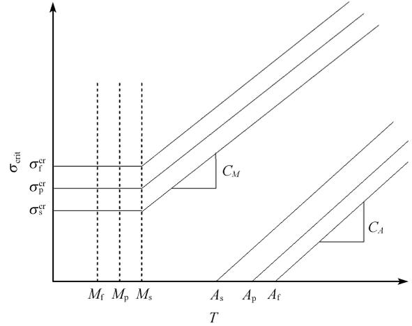
**Figure 4** The new relationship of phase transformation critical stresses and temperature.
