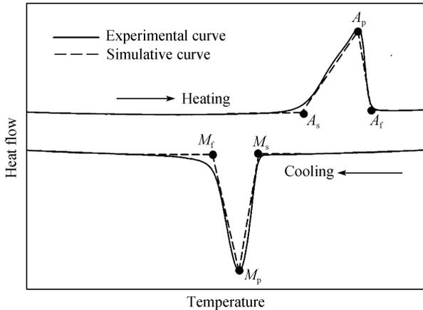
Figure 2 The curve of DSC test and its simulation.
