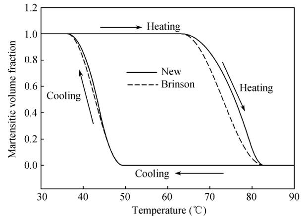
**Figure 5** Martensitic volume fraction-temperature curves.
