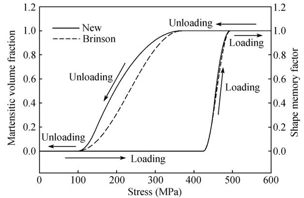
**Figure 6** Martensitic volume fraction/shape memory factor-stress curves.
