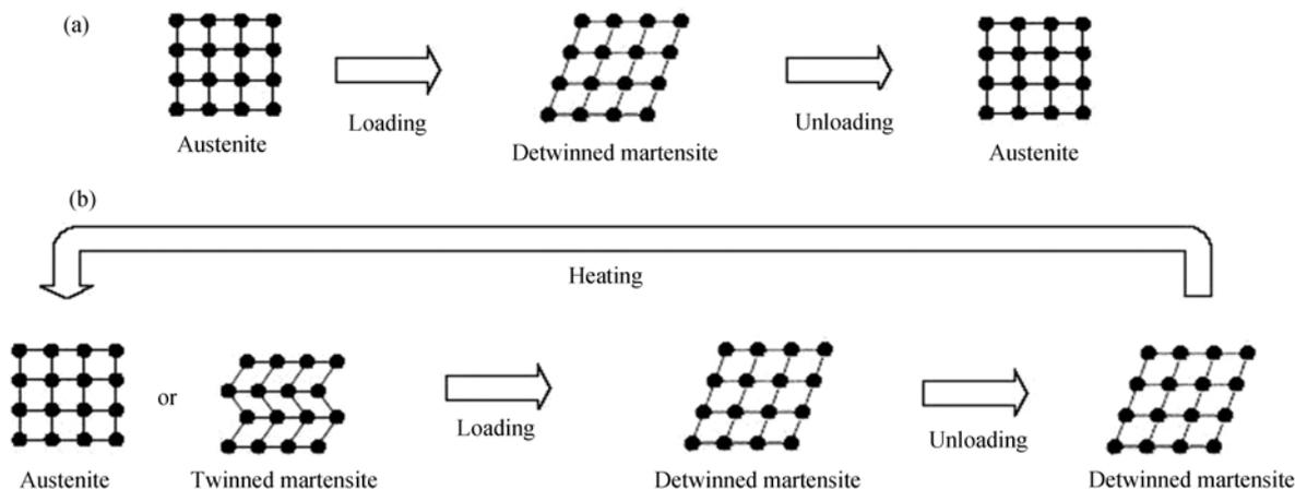
**Figure 1** The microscopic mechanism of shape memory effect of SMA. (a) The microscopic mechanism of conventional super elasticity of SMA; (b) the microscopic mechanism of conventional shape memory effect of SMA.
