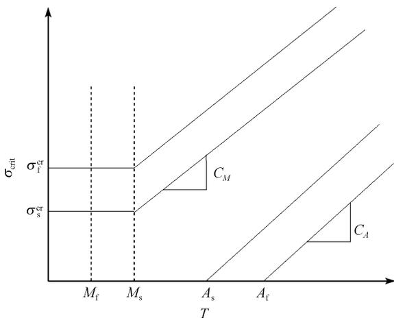
**Figure 3** The Brinson's relationship of phase transformation critical stresses and temperature.<sup>[6]</sup>
