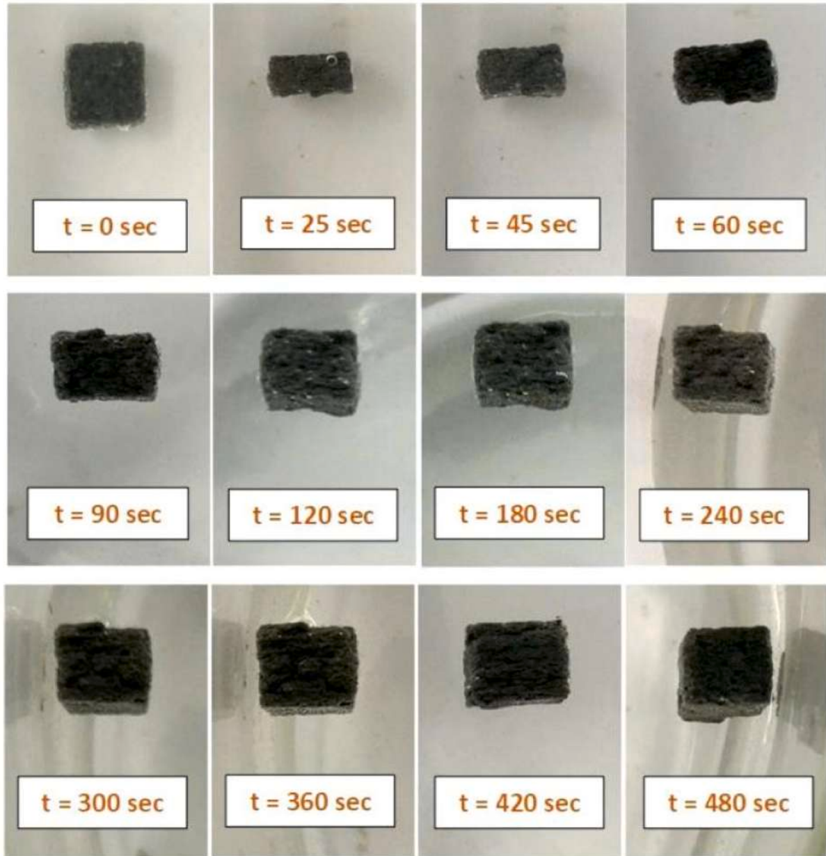
Fig. 27. The shape recovery process of SMPU/Tungsten composite sample [129].
