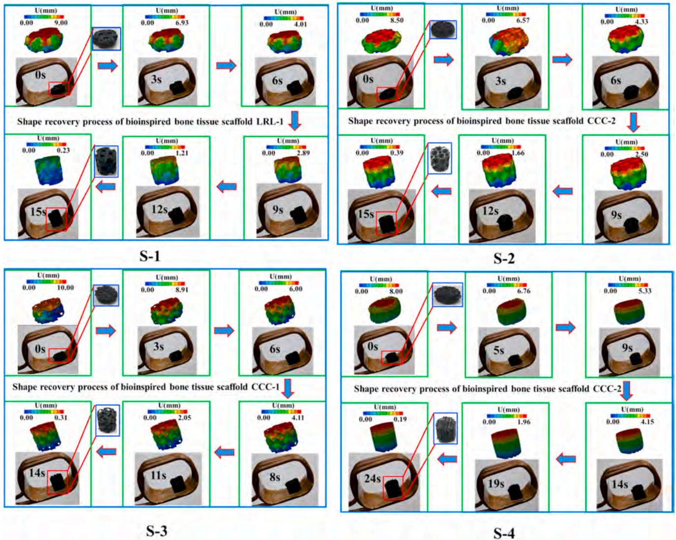
Fig. 6. Illustration of the shape recovery process by FEA and experiment for S-1, S-2, S-3 and S-4 (a) S-1 (b) S-2 (c) S-3 (d) S-4.
