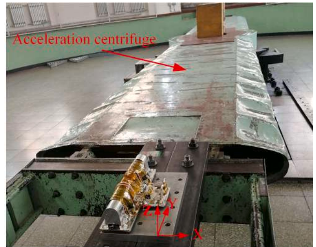
Fig. 12. Acceleration test of the SMPC-FSAS in the stowed state [33].
