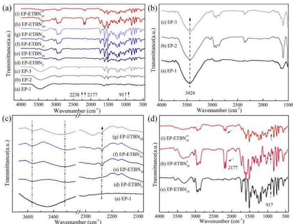
Fig. 2. FTIR spectra of SMEPs: (a) SMEPs. (b), (c) and (d) zoom in part of (a).
