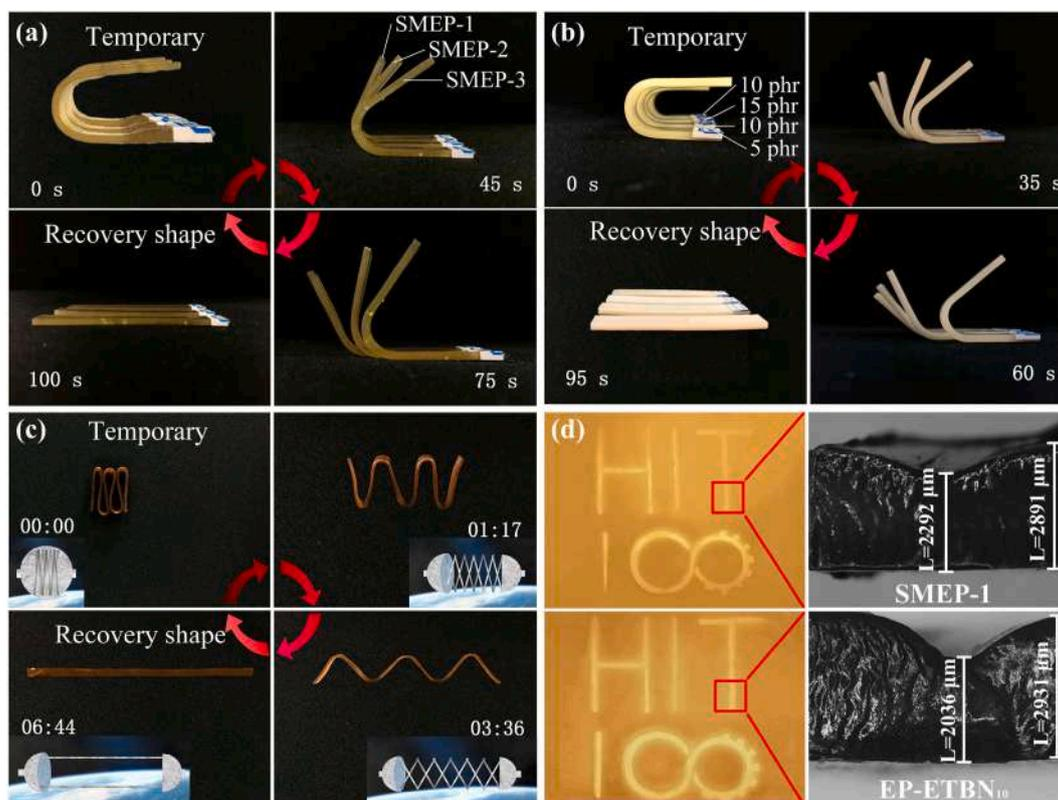
Fig. 7. Characterization of the shape-memory behavior of systems: (a) and (b) Shape recovery process, (c) Simulation process of space capsule, (d) Engrave “the 100th Anniversary”.
