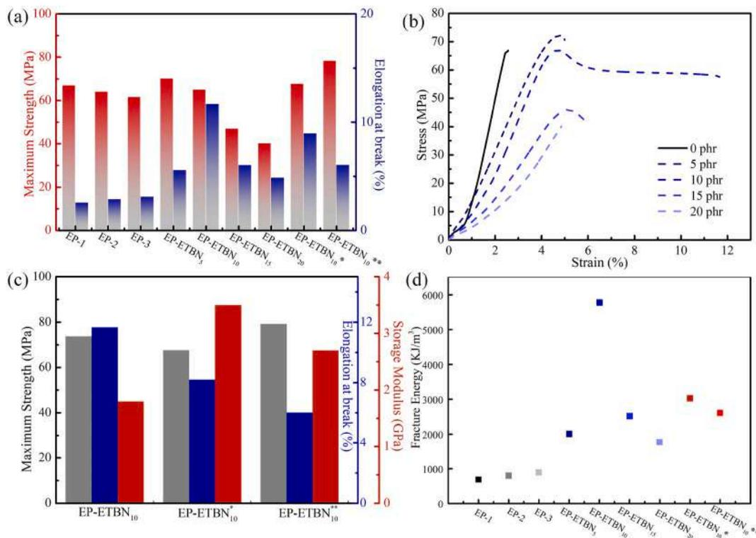
Fig. 4. Mechanical properties of systems: (a) and (b) results of a tensional test at room temperature. (c) typical stress-strain curves at room temperature. (d) toughness at room temperature.
