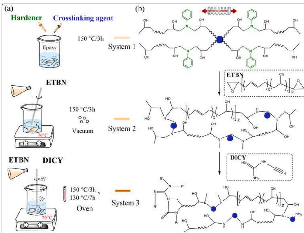
Fig. 1. (a) Preparation process of systems. (b) Reaction process for preparing systems.
