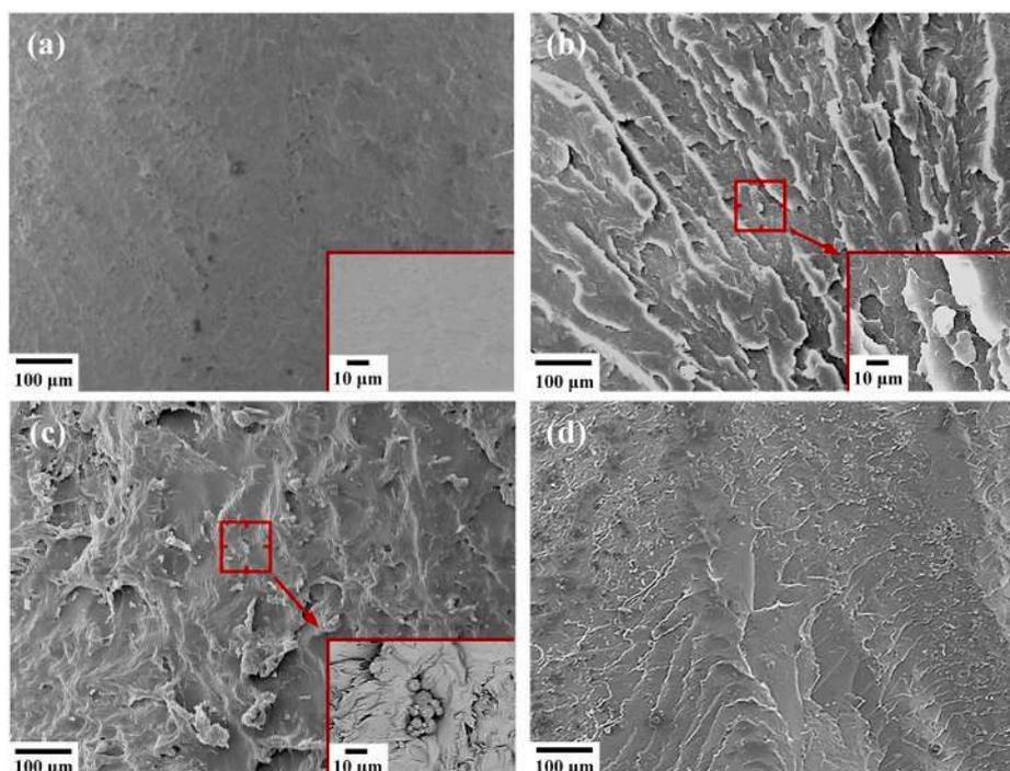
Fig. 5. SEM micrographs of the fracture surface for systems: (a) pure ESMP, (b) EP-ETBN<sub>5</sub>, (c) EP-ETBN<sub>10</sub> and (d) EP-ETBN<sub>10</sub>\*\*.
