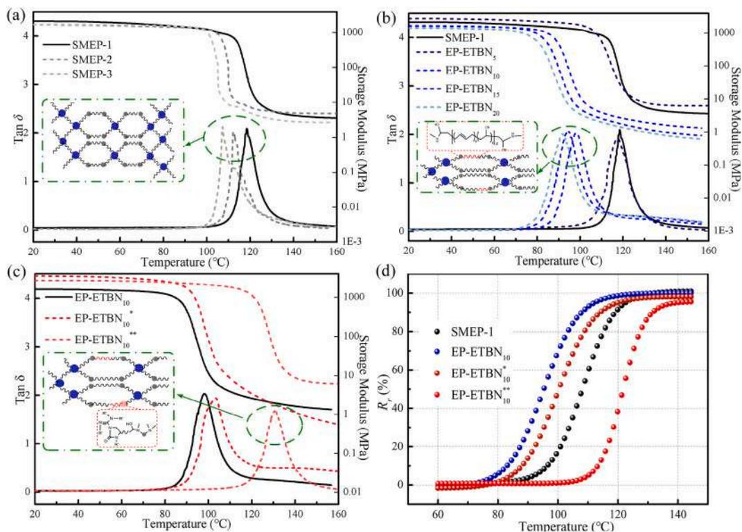
Fig. 6. (a), (b), and (c) The DMA curves of systems. (d) The shape recovery ratio of System 3.
