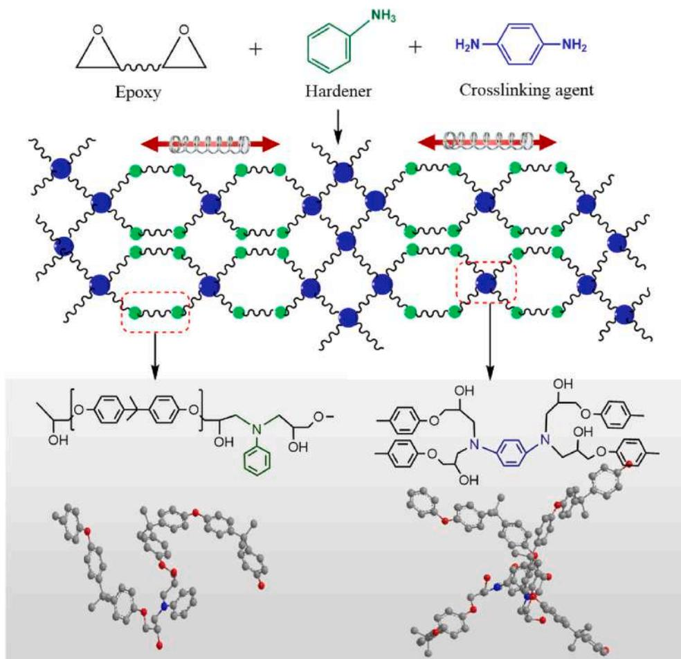
**Scheme 1.** Schematic illustration of the regular and uniform cross-linked network of SMEP.
