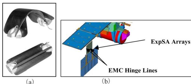
**Figure 10.** Tembo<sup>®</sup> EMC Hinge, (a) the images of EMC Hinge in packaged and deployed configurations, (b) TacSat-2 experiment [65].
