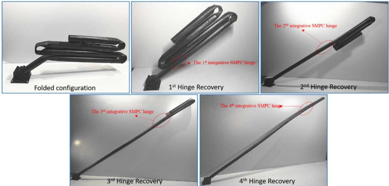
Figure 18. Deployment process of the self-deployable tube [38].
