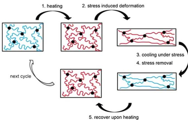
**Figure 2.** The molecular mechanism of the SMP, • crosslinking points; — low mobility molecular chains below  $T_m/T_g$ ; — high mobility molecular chains above  $T_m/T_g$  [94].
