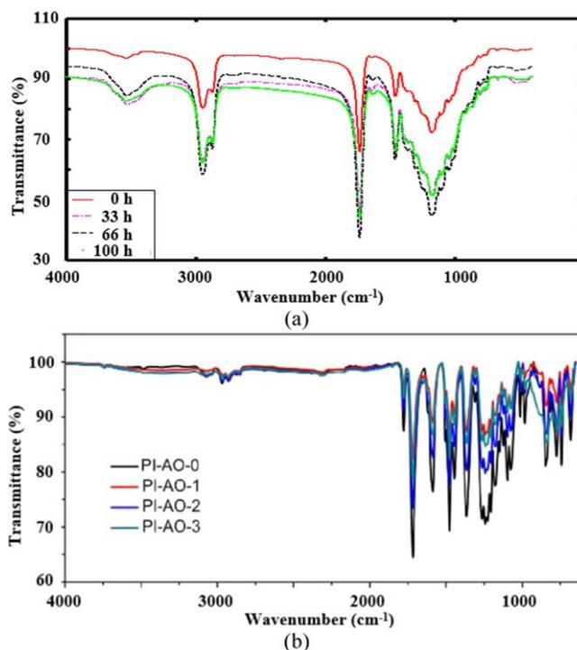
**Figure 9.** FTIR spectra of materials before and after AO irradiation, (a) SMPEP [143], (b) SMCTPI [145].
