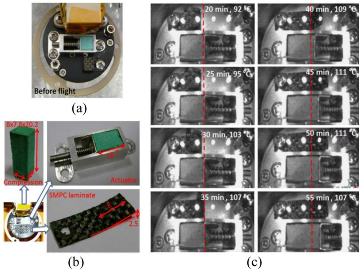
Figure 15. The Ribes\_Foam2 experiment, (a) the samples and experimental unit before flight, (b) size of samples after flight, (c) images of recovery during heating on-board [71].
