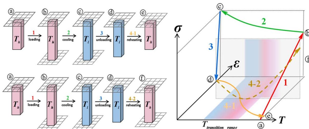
**Figure 1.** Schematics of shape recovery processes, (a) free recovery process, (b) constraint recovery process, (c) the temperature-strain-stress curves at different recovery process (1. Loading at high temperature (above  $T_g$ ), 2. Cooling with external constraints, 3. releasing the constraints, 4-1 free recovery process, 4-2 constraint recovery process).
