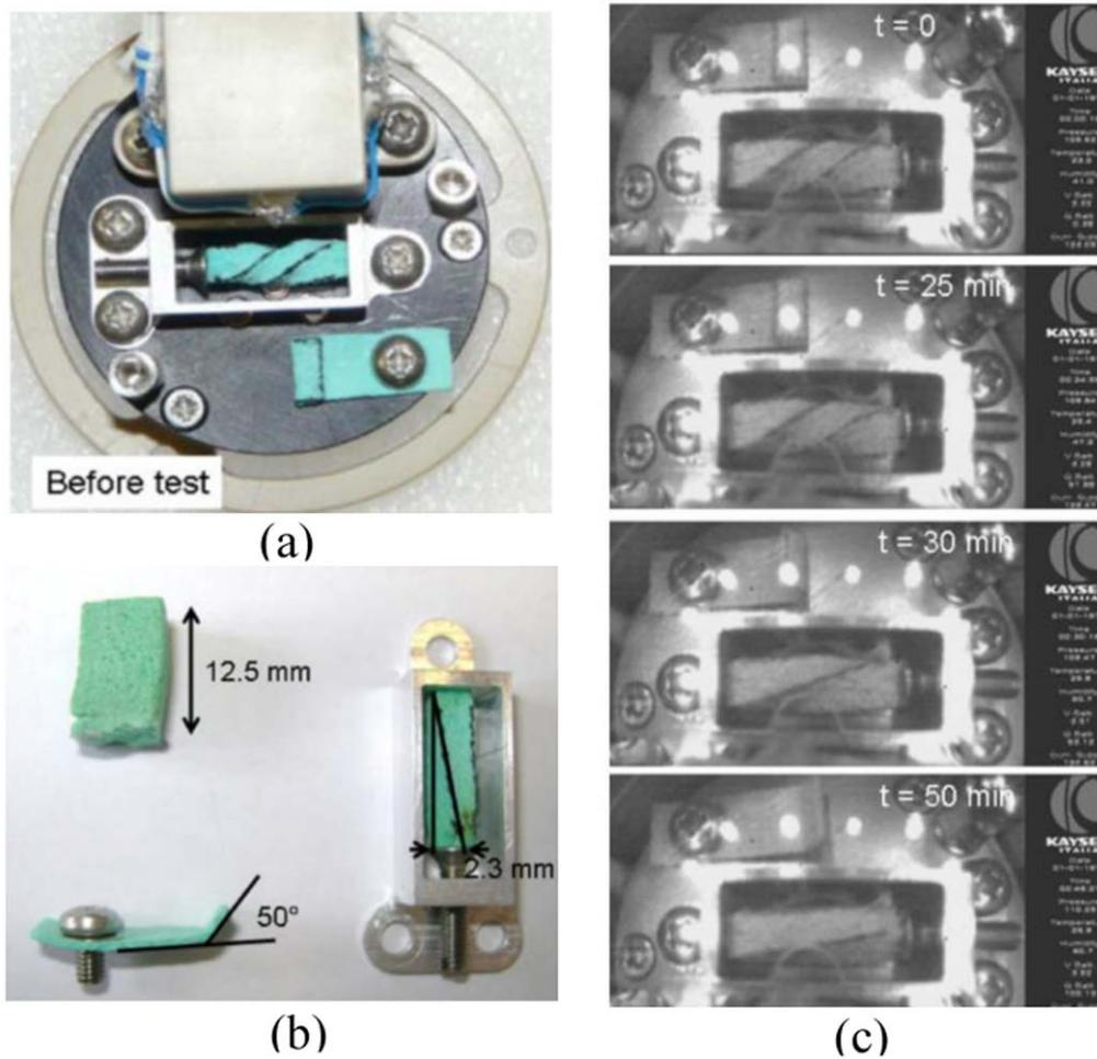
Figure 13. The I-FOAM experiment, (a) initial shape of samples, (b) final shape of samples, (c) progress of recovery in the ISS [70].
