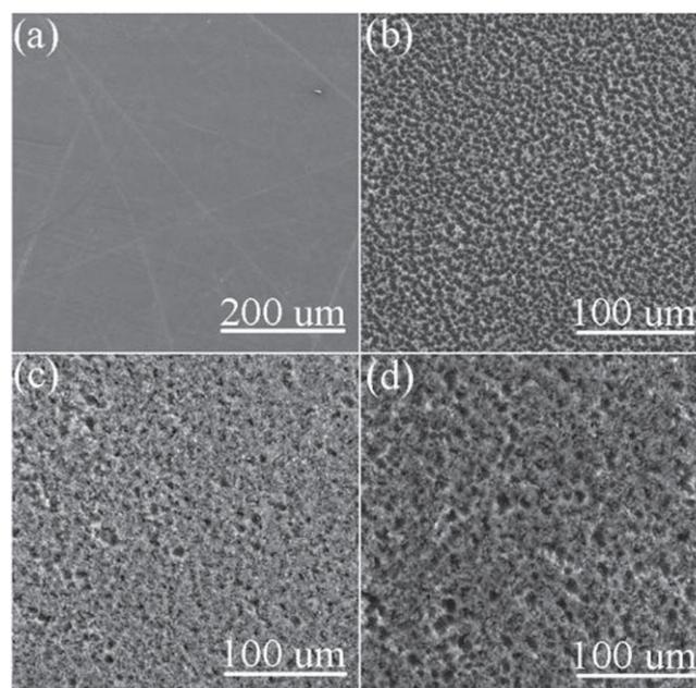
**Figure 8.** Surface morphologies of SMCTPI samples exposed to different AO radiation doses, (a) 0, (b)  $3 \times 10^{21} \text{ O cm}^{-2}$ , (c)  $6 \times 10^{21} \text{ O cm}^{-2}$ , (d)  $10 \times 10^{21} \text{ O cm}^{-2}$  [145].
