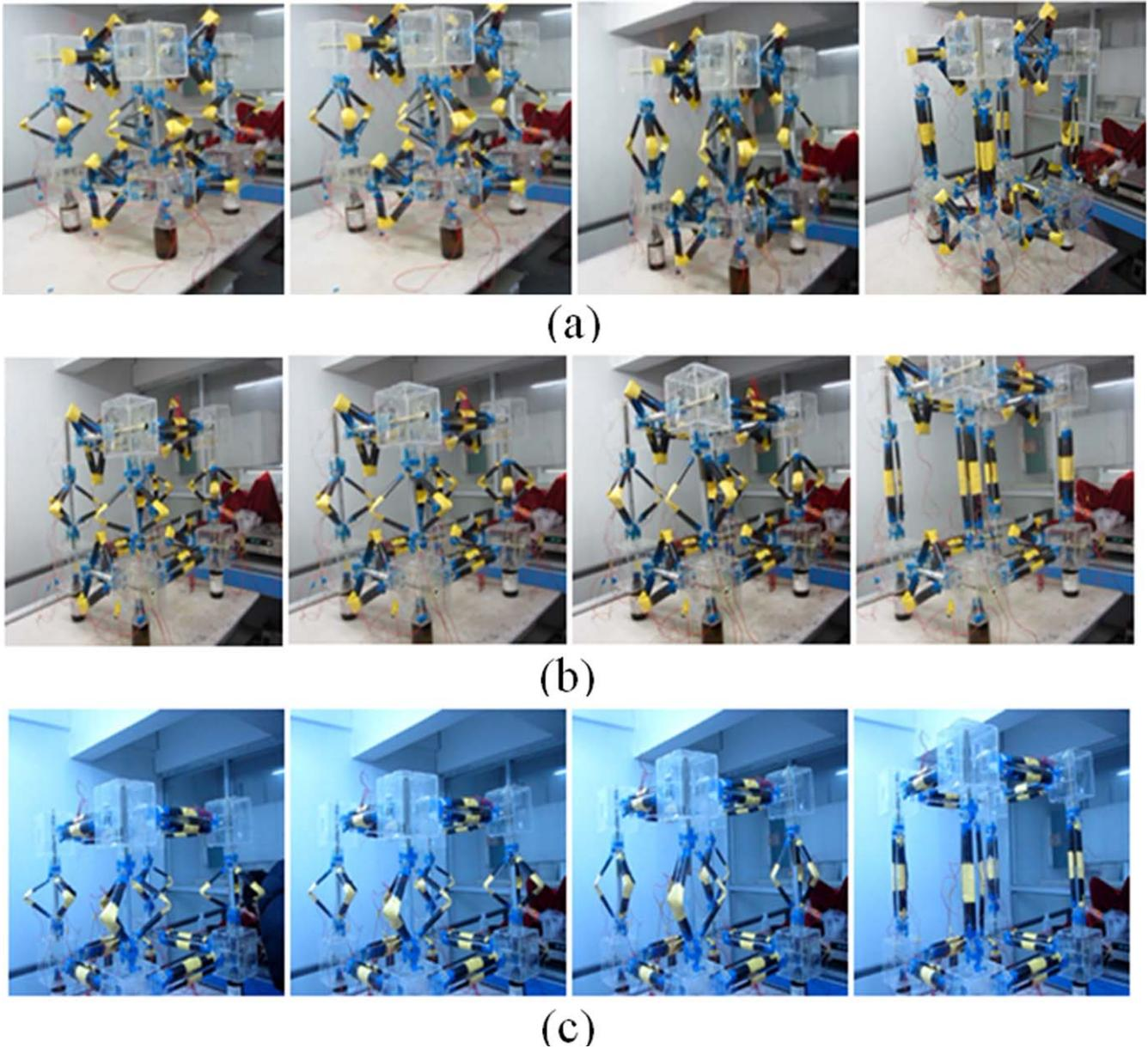
**Figure 20.** The deployment process of the cubic deployable support structure, in the first direction, (b) in the second direction, (c) in the third direction [82].
