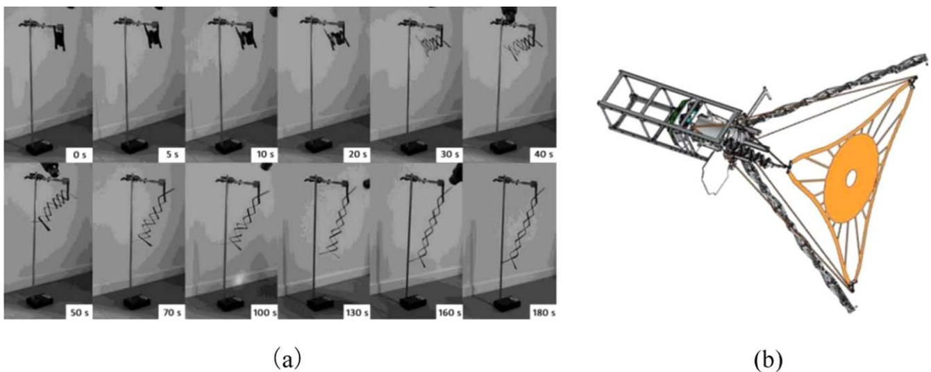
Figure 19. Repeated X-shape mast based on SMPC, (a) deployment process, (b) potential application at deployable membrane telescope for a CubeSat [166, 167].
