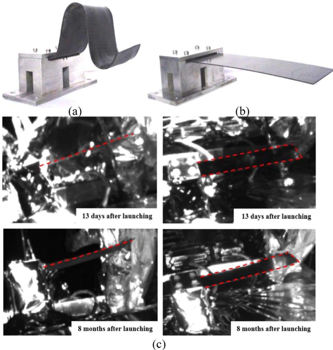
**Figure 16.** Mission SMS-I, (a) the packaged configuration, (b) the deployed configuration, (c) orbital images 13 d and 8 months after launching [157].
