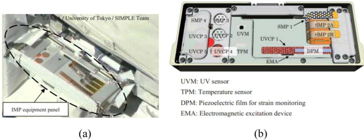
Figure 14. Inflatable Material Panel (IMP), (a) overall view of IMP during spaceflight, (b) specimen layout of IMP [156].
