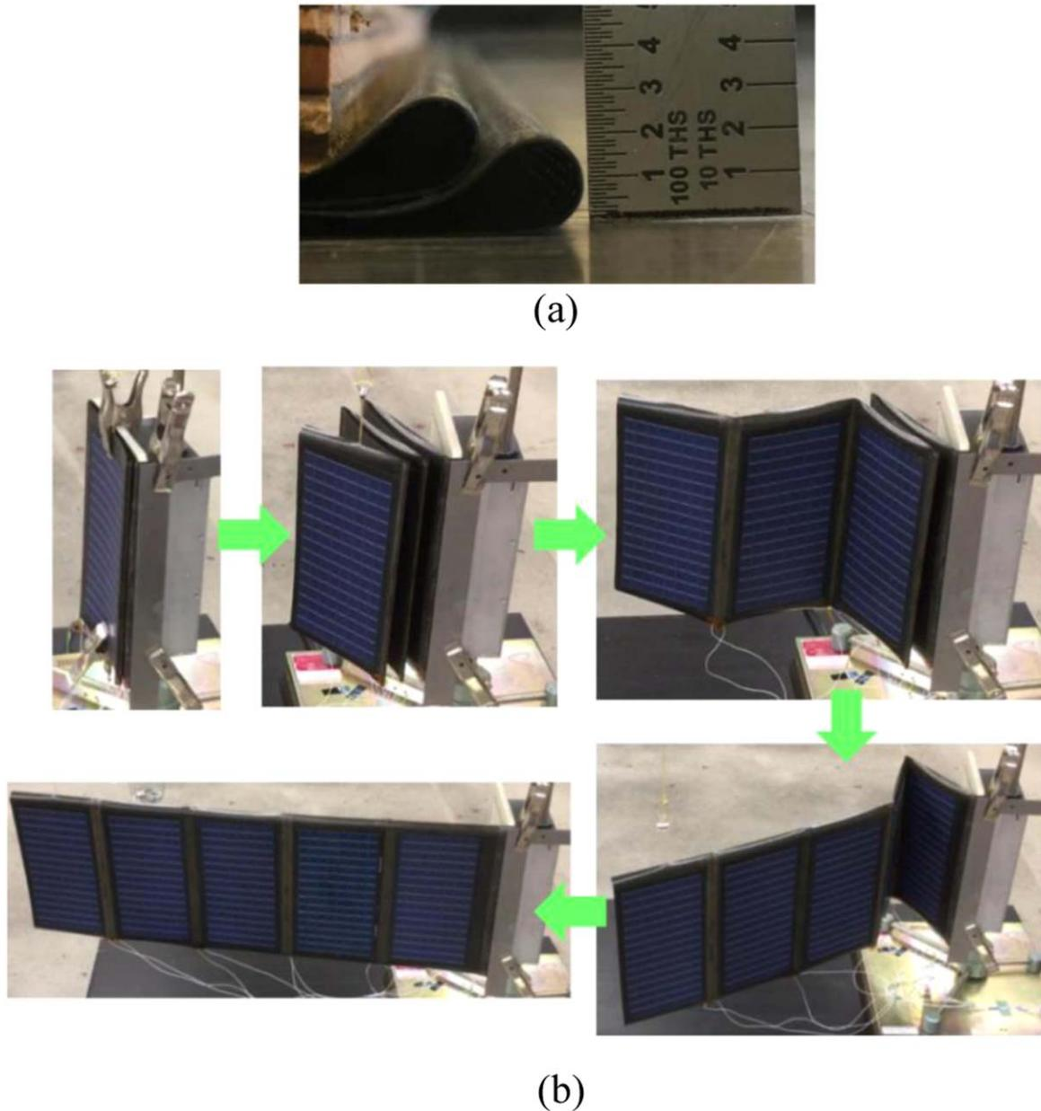
**Figure 24.** Composite lightweight array using shape-memory polymer (CLASP), (a) nested (P-folded) hinge-line, (b) deployment process of CLASP on a mock 6U CubeSat [164].
