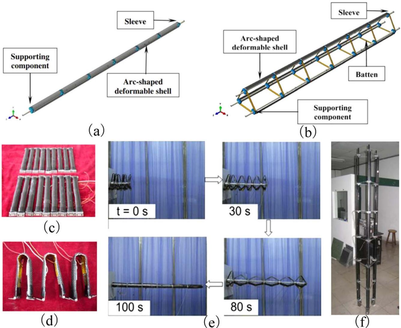
**Figure 17.** Two kinds of deployable trusses, (a) schematic of the three-longeron beam, (b) schematic of the three-longeron truss, (c) unfolded SMPC laminates, (d) folded SMPC laminates, (e) the deployment process of the three-longeron beam, (f) the modal of the three-longeron truss [50, 165].
