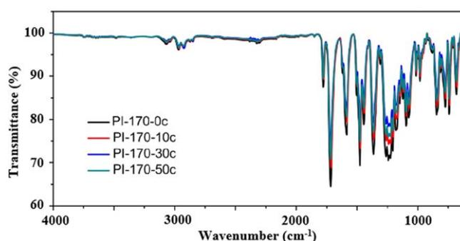
**Figure 5.** FTIR spectra of SMCTPI before and after temperature cycling [145].
