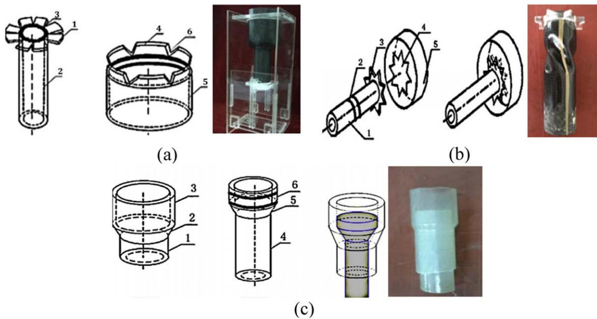
**Figure 22.** Smart release devices, (a) the ‘Lotus’ device, (b) the ‘Eight paws’ device, (c) the ‘Bamboo’ device [28].
