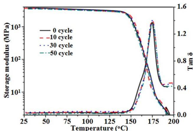
**Figure 4.** DMA curves of the SMCTPI before and after temperature cycling [145].
