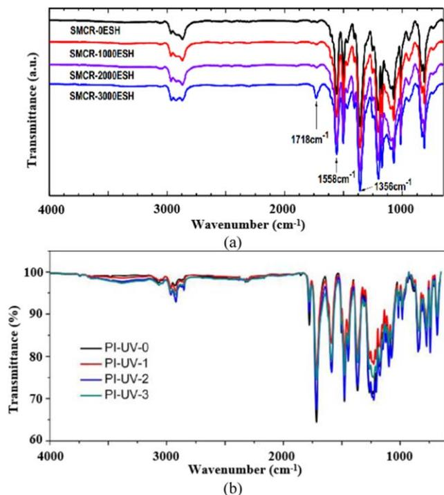
**Figure 7.** FTIR spectra of materials before and after UV radiation, (a) SMP-CRIV [142], (b) SMCTPI [145].
