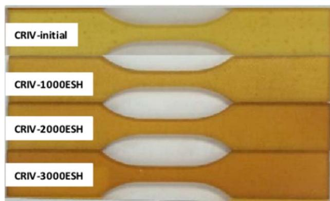
**Figure 6.** Images of SMP-CRIV samples before and after UV radiation [142].
