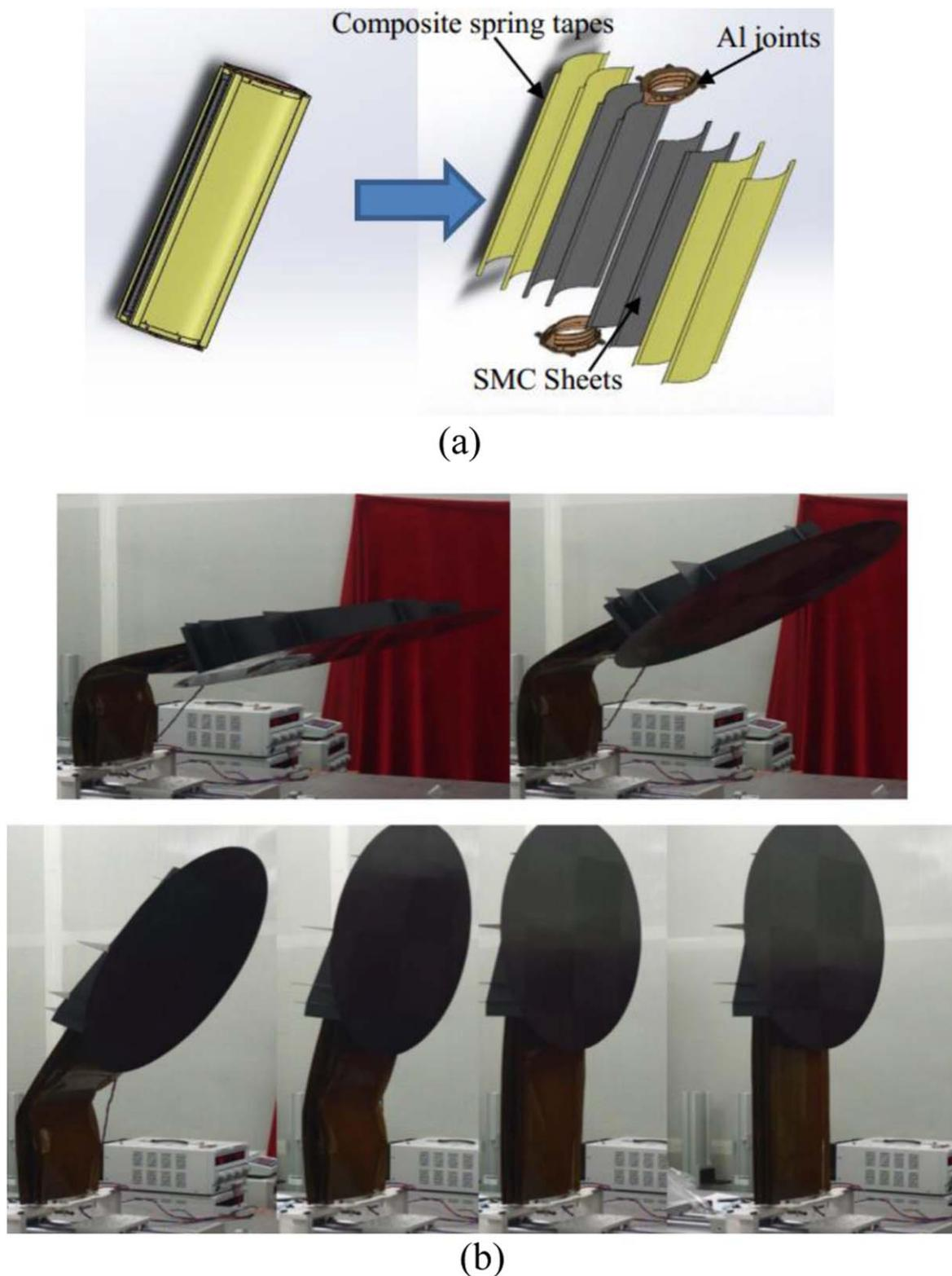
**Figure 23.** Space deployable mechanism (SDM), (a) configurations of SDM, (b) the deployment process [162].
