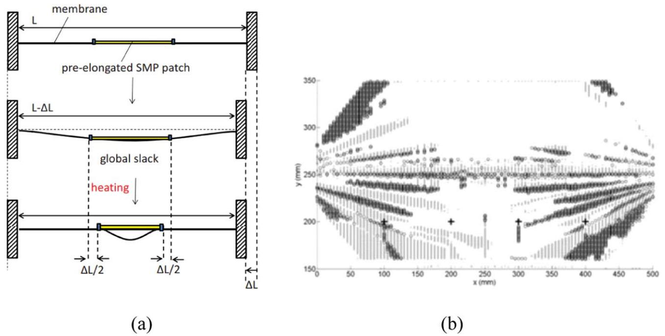
**Figure 21.** SMP films for wrinkled/slack control, (a) schematic of the shape control concept by attaching a SMP film on the membrane’s surface, (b) comparison of the measured out-of-plane displacement before and after the SMP film wrinkle control [163].
