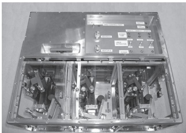
**Figure 11.** EMC hinge flight unit in International Space Station (ISS) environment [65].
