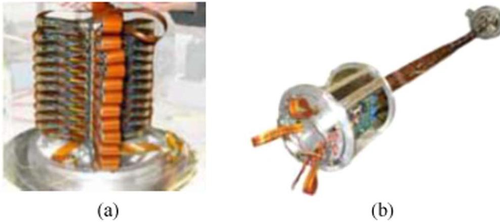
Figure 12. The proposed FalconSat-3 deployable gravity gradient boom, (a) the packaged configuration, (b) the deployed configuration [65].
