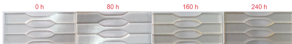
Figure 3. The color of epoxy-based SMP before and after UV radiation.
