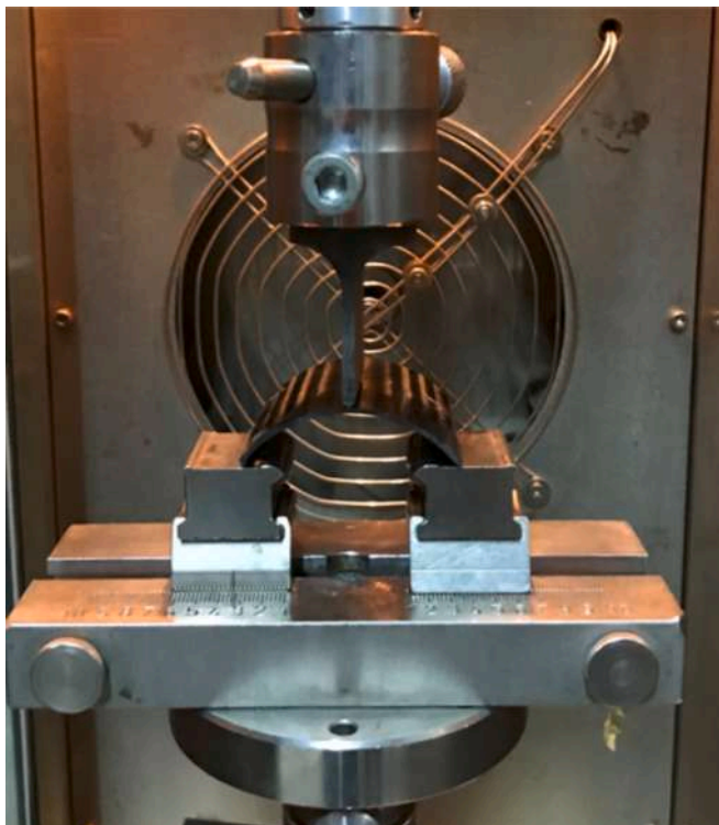
Fig. 2. Three-point bending test.
