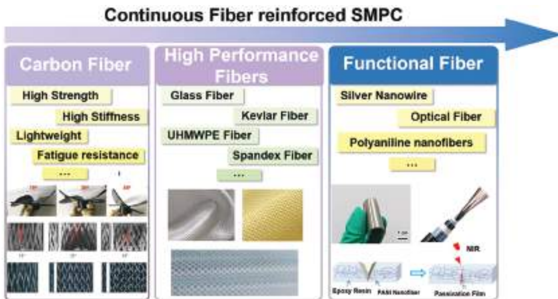
Figure 12. The evolution of SMPC reinforced with continuous fibers.
